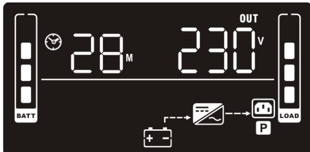
In case of a power failure or when the input voltage is beyond the acceptable range, the UPS changes to battery mode to keep powering the connected loads. An alarm will keep sounding every 5 seconds during battery mode.
