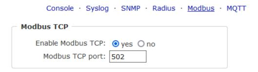
Enable Modbus TCP: Enables Modbus TCP support.
