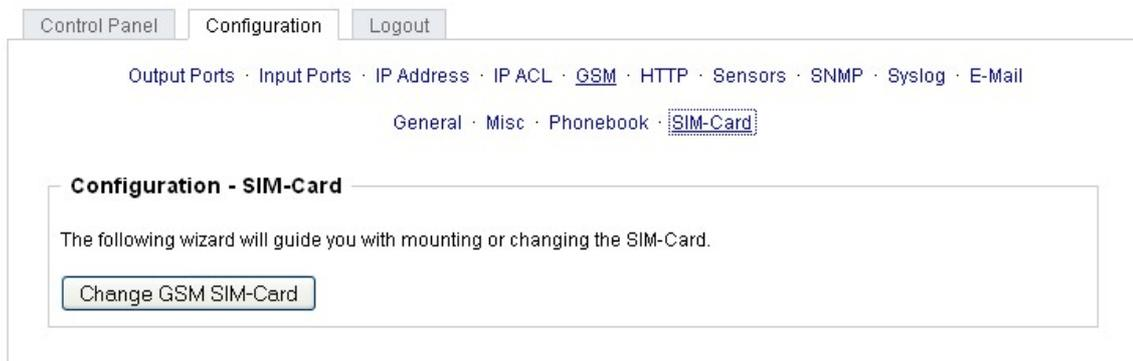
To enter a new SIM card, please press the button "Change GSM SIM-card".
