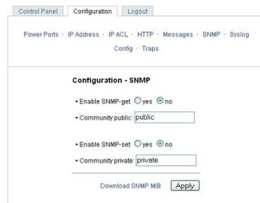
The screenshot shows a web interface with a navigation bar at the top containing 'Control Panel', 'Configuration', and 'Logout'. Below the navigation bar is a breadcrumb trail: 'Power Ports · IP Address · IP ACL · HTTP · Messages · SNMP · Syslog'. The main content area is titled 'Configuration - SNMP' and contains the following settings:
