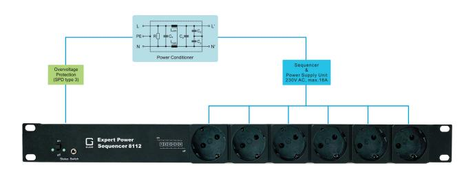
This layout is valid for Expert Power Sequencer 8112-4 and also 8112-2 with 6 IEC C13 instead of safety sockets on the front panel.
