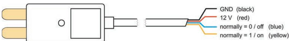
In the event of flooding, when the two electrodes are wetted by liquid, the blue wire is connected to GND and the yellow is disconnected. In the dry state it is the other way around: The yellow cable is connected to GND and the blue is disconnected.
